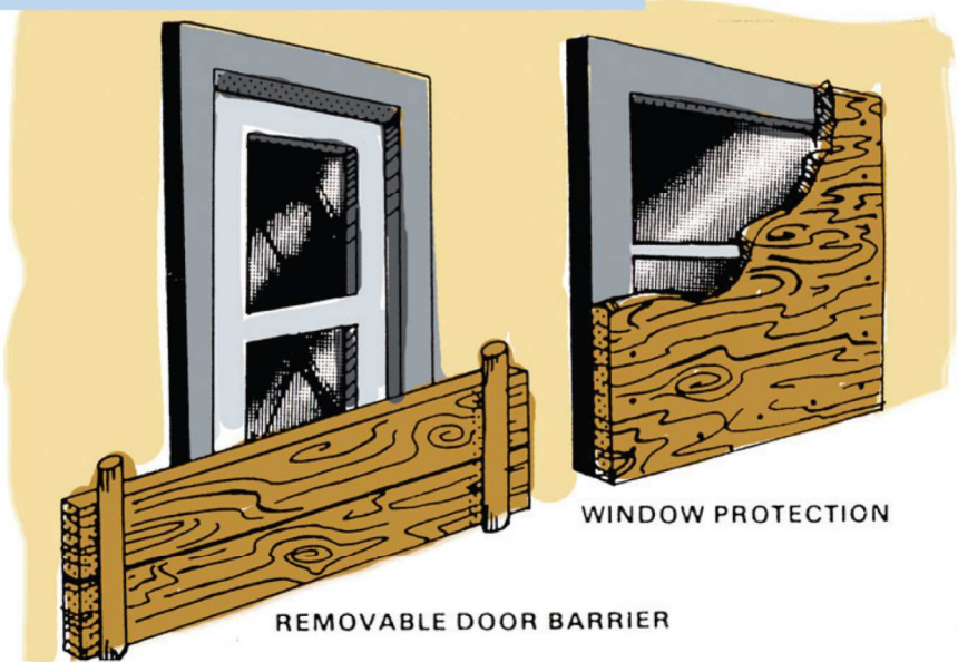
Figure 14: Typical Window/Door Protection - Use of plywood or lumber can help protect windows and doors from damage.
